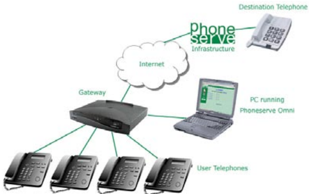
Figure 1. Minimum Setup with a direct DSL connection
