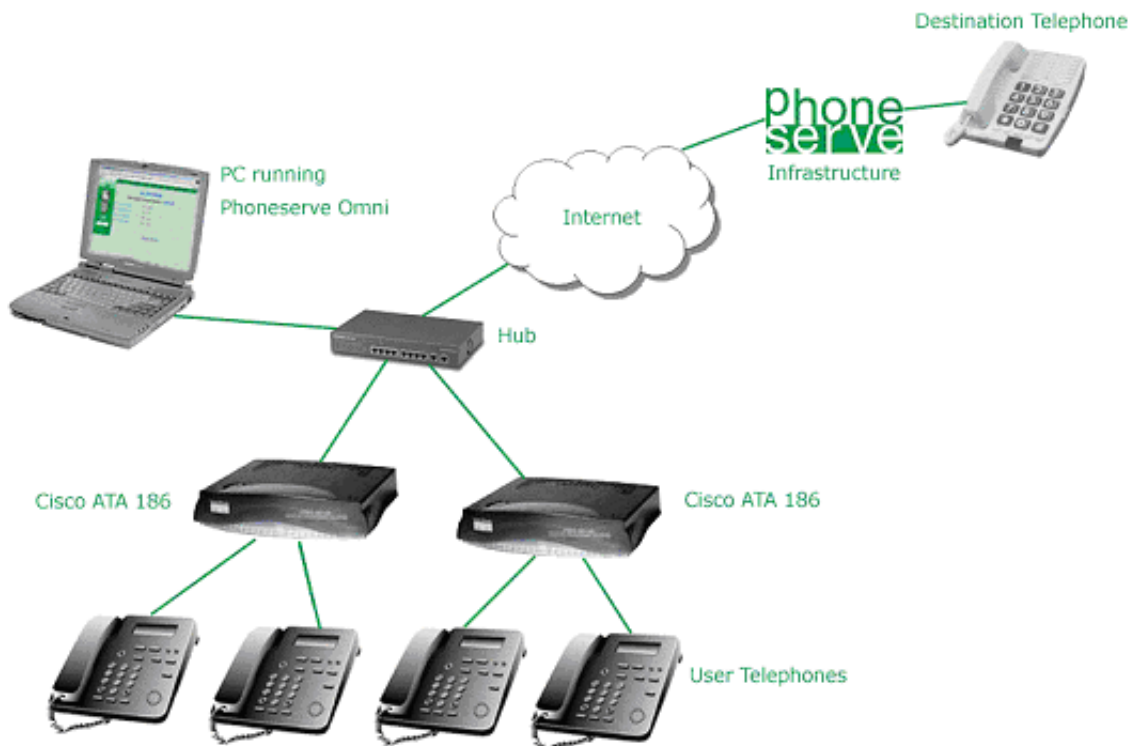
Figure 1. Example of a ATA186 set-up using an existing network (LAN)
